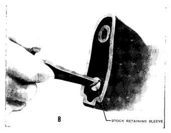
Figure 78. Replacing the stock retaining sleeve.
