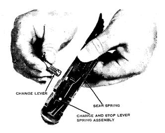
Figure 49. Replacing the change lever.
