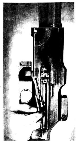
Figure 7. Removing the trigger guard retaining pin assembly.
