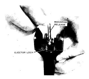
Figure 60. Replacing the magazine release.
