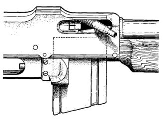
Figure 116.4. (Added) Failure to eject.
