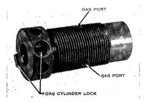
Figure 110. Gas cylinder assembly.
