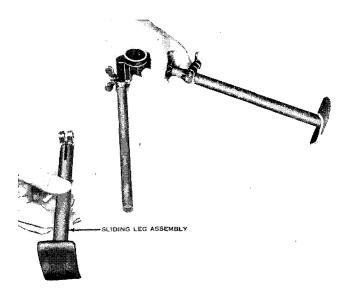
Figure 83. Removing the sliding leg assembly.
