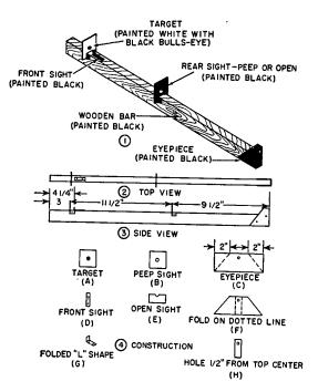
Figure 178. Sighting and aiming bar.
