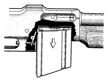
Figure 112. (Superseded) Failure to feed.
