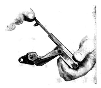
Figure 25. Replacing the firing pin.
