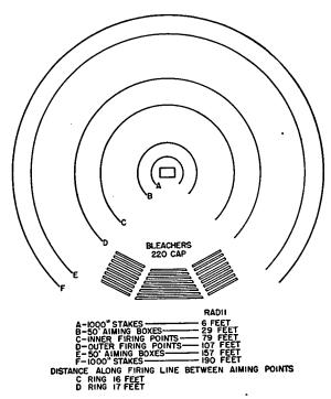
Figure 159. Layout of the preparatory marksmanship field, circular type (temporary).
