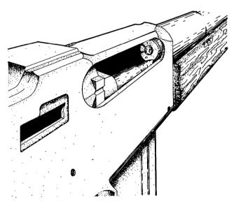
Figure 116.2. (Added) Failure to extract due to broken extractor spring.
