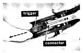
Figure 40. Removing the trigger and connector.
