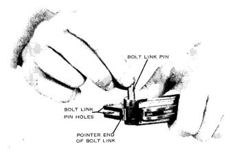
Figure 24. Replacing the bolt link and bolt link pin.
