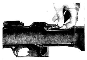
Figure 93. Replacing the extractor.
