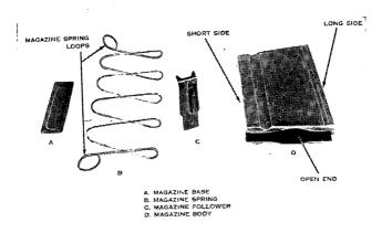
Figure 88. Layout of parts of the magazine group.
