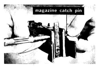
Figure 37. Removing the magazine catch pin.
