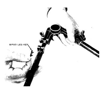
Figure 82. Removing the bipod leg key.
