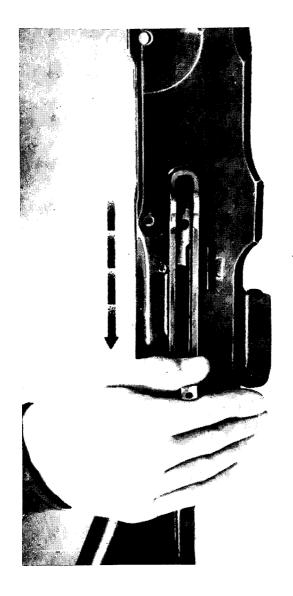
Figure 14. Removing the operating handle.
