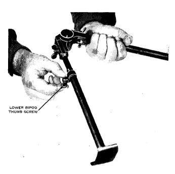
Figure 81. Removing the lower bipod thumb screw (wing nut).
