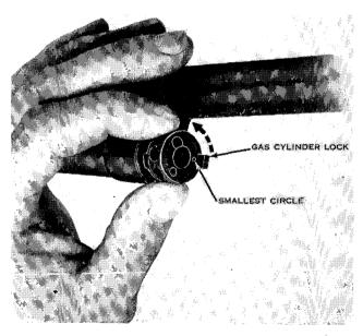
Figure 111. Adjustment of gas cylinder on small port.
