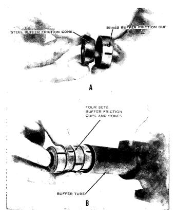
Figure 75. Replacing the four sets of brass buffer friction cups and steel buffer friction cones.
