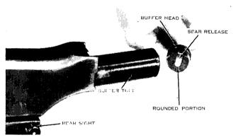
Figure 74. Replacing the buffer head assembly.
