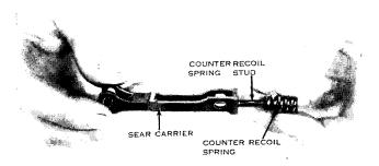
Figure 50. Assembling the sear carrier and counterrecoil spring.
