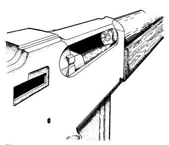
Figure 1163. (Added) Failure to extract due to dirty or pitted chamber, or faulty ammunition.
