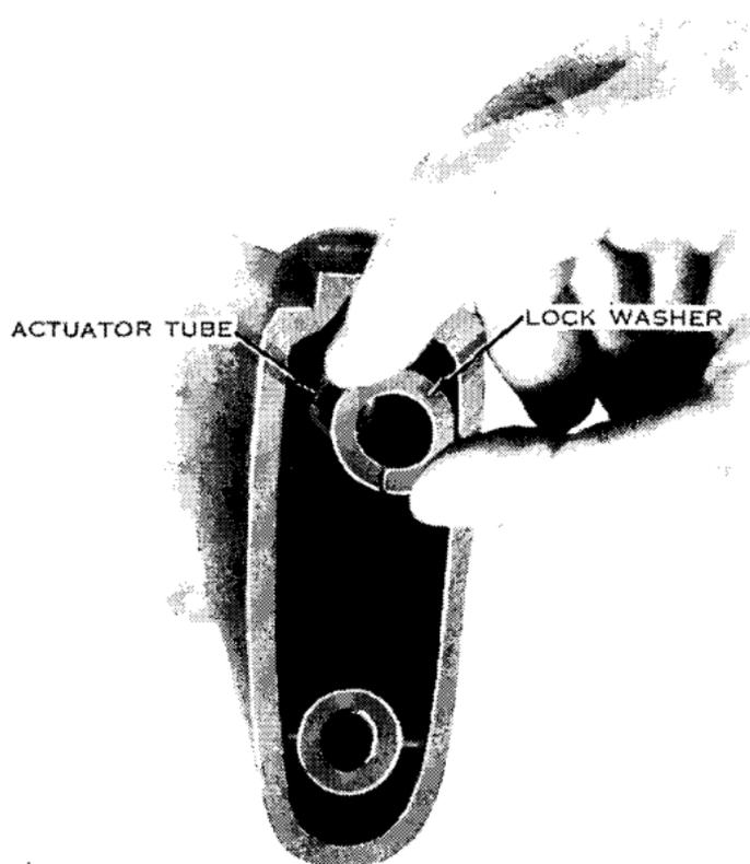
*Figure 76. Replacing the lock washer.*
