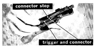
Figure 57. Replacing the trigger and connector.
