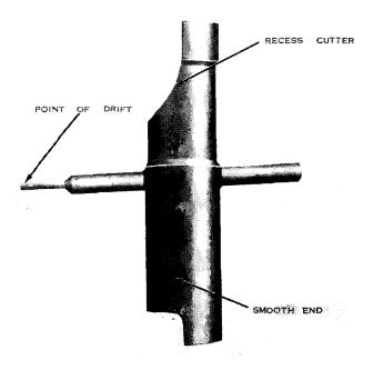
Figure 117. Gas cylinder cleaning tool.
