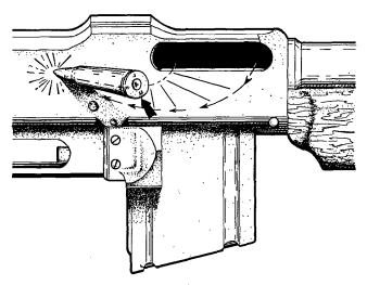
Figure 116.1. (Added) Failure to fire due to excessive friction, a weak recoil spring, or faulty ammunition.
