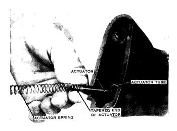
Figure 77. Replacing the actuator and actuator spring.
