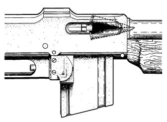
Figure 114. (Superseded) Double chambering.
