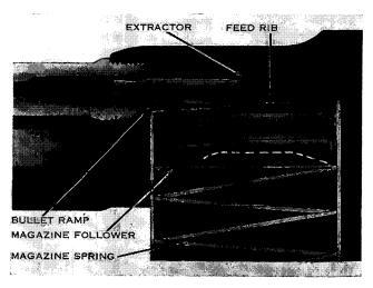
Figure 94. (Superseded) Chambering.
