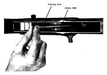
Figure 90. Replacing the firing pin.
