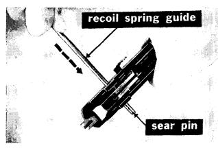
Figure 41. Removing the sear pin.
