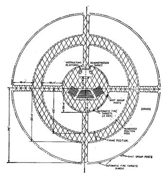
Figure 160. Layout of two-company circular preparatory marksmanship field (permanent).
