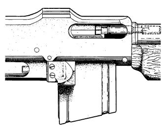
Figure 115. (Superseded) Failure to chamber due to ruptured cartridge.
