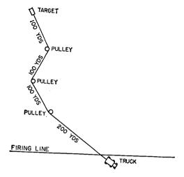
Figure 168. Layout for a moving target range.
