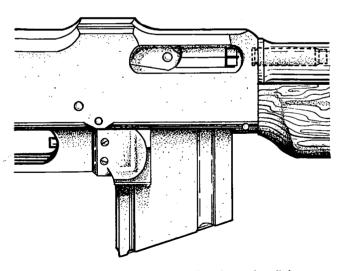
Figure 116.5. (Added) Failure to eject due to insufficient gas.
