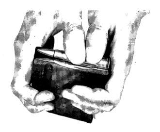
Figure 107. Loading single rounds into the magazine.
