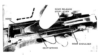
Figure 59. Replacing the sear spring. 947041°—51—5
