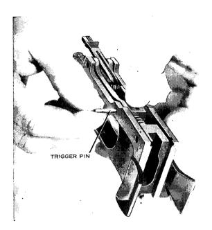
Figure 58. Replacing the trigger pin.
