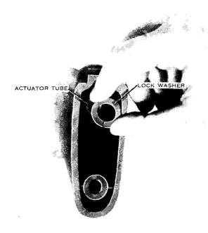
Figure 76. Replacing the lock washer.
