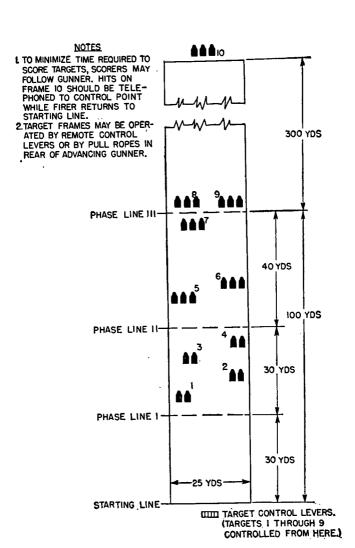
Figure 166. Layout for automatic rifle transition range for firing table VIII.
