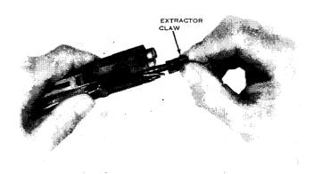
Figure 23. Replacing the extractor and extractor spring.
