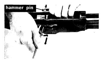
Figure 29. Replacing the hammer pin.
