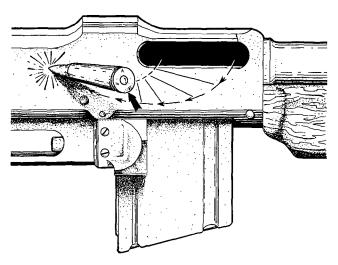
Figure 116. (Superseded) Failure to fire due to broken firing pin.
