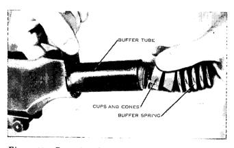
Figure 69. Removing the buffer spring and the four sets of brass buffer friction cups and steel buffer friction cones.
