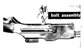
Figure 26. Replacing the bolt assembly.
