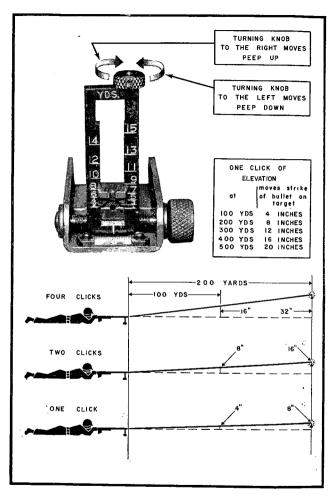
Figure 144. Elevation rule.
