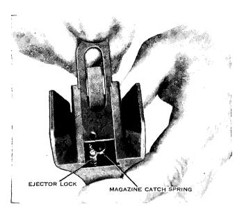
Figure 63. Replacing the ejector and magazine catch spring.
