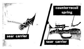
Figure 43. Unscating the sear carrier and removing the counterrecoil spring.
