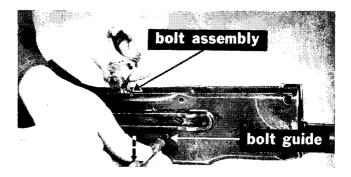
Figure 17. Removing the bolt assembly.
