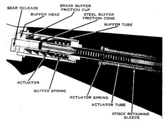
Figure 97. The buffer and rate reducing group.
