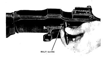
Figure 89. Allowing the bolt assembly to buckle.
