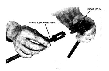
Figure 85. Removing the bipod leg assembly.
