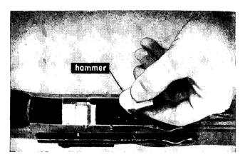
Figure 15. Removing the hammer.
