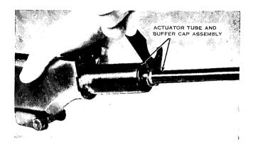
Figure 68. Removing the actuator tube and buffer cap assembly.
