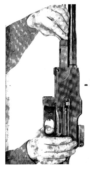
Figure 6. Allowing the operating parts to go forward.
