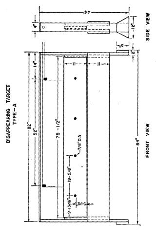
Figure 161. Disappearing target, type A.
