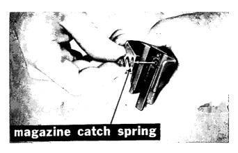
Figure 36. Removing the magazine catch spring.
