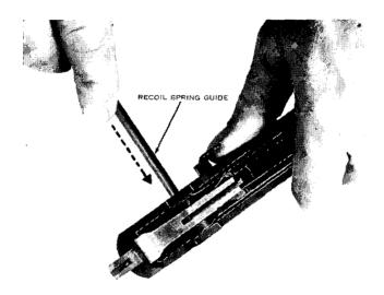
Figure 54. Alining the sear pin holes.
