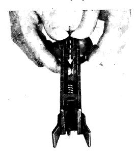
Figure 51. Replacing the sear carrier (first method).
