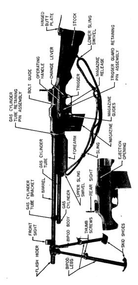
Figure 1. Browning Automatic Rifle, Caliber .30, M1918A2.
