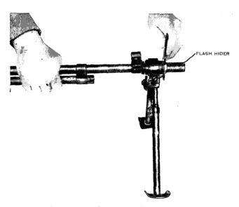
Figure 79. Removing the flash hider.
