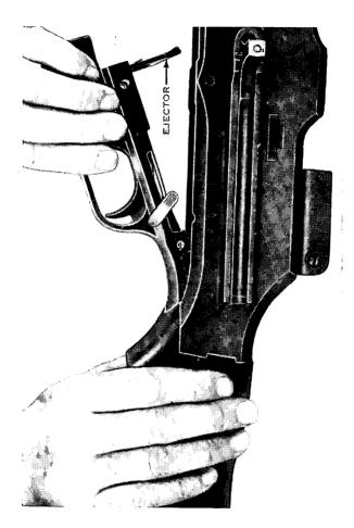
Figure 8. Removing the trigger group.
