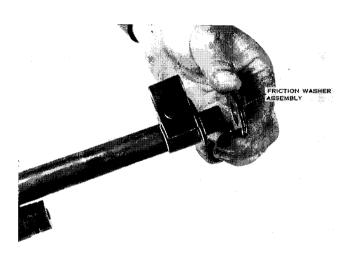
Figure 80. Removing the friction washer assembly.
