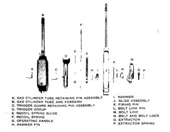
Figure 21. Layout of parts of the operating group.
