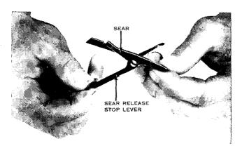
Figure 53. Assembling the sear and sear release stop lever.
