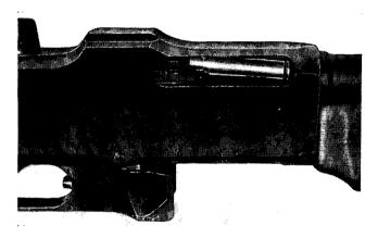
Figure 91. The operating parts held in place by the empty cartridge case.
