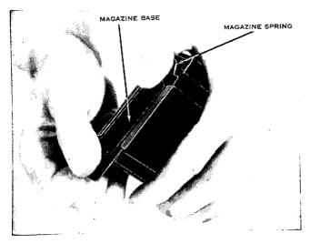
Figure 87. Removing the magazine base.
