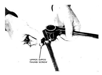
Figure 84. Removing the upper bipod thumb screw (wing nut).
