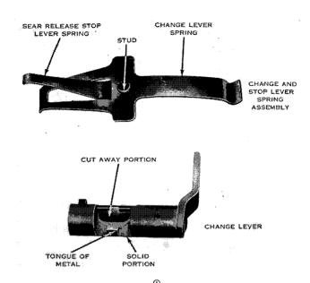
Figure 98. Trigger group parts.
