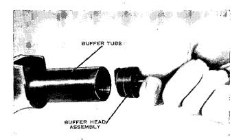
Figure 70. Removing the buffer assembly.
