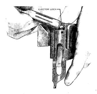
Figure 64. Seating the ejector.
